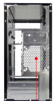
Rear Fan: 80x80 mm x1 or 90x90 mm x1 (Optional)
