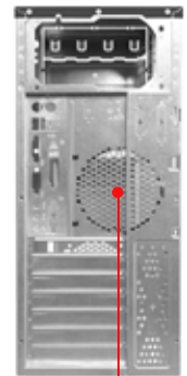
Rear Fan: 80x80 mm x 1 or 92x92 mm x 1
