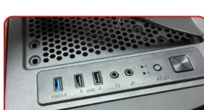
USB 3.0 x1 / USB2.0 x 2 / HD Audio In/Out / LED light switch on the top
